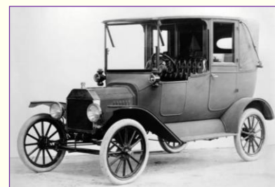
Source 51. Ford Model T of 1908, the first car to be produced by mass production
